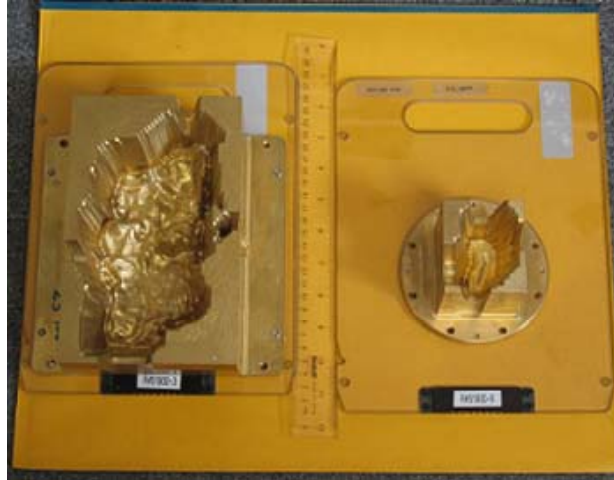
Figure 19. Two modulators from •Decimal mounted on the Siemens coded trays. One of the large compensators (11.3 kg) from the initial 7-field plan that did not require extensive blocking within the field is shown next to one of the 7-field IMRT modulators for prostate (1.8 kg).
